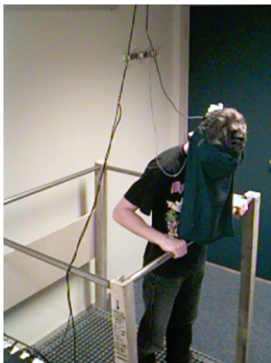
Figure 1: Setup used for the experiments. The subject is wearing the HMD with a piece of cloth to mask the real environment and is standing on a metal grid suspended a few inches above the ground, clutching the railing.
